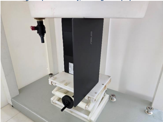
Testing Setup for Extremity, Left Edge of Laptop at 0 mm
