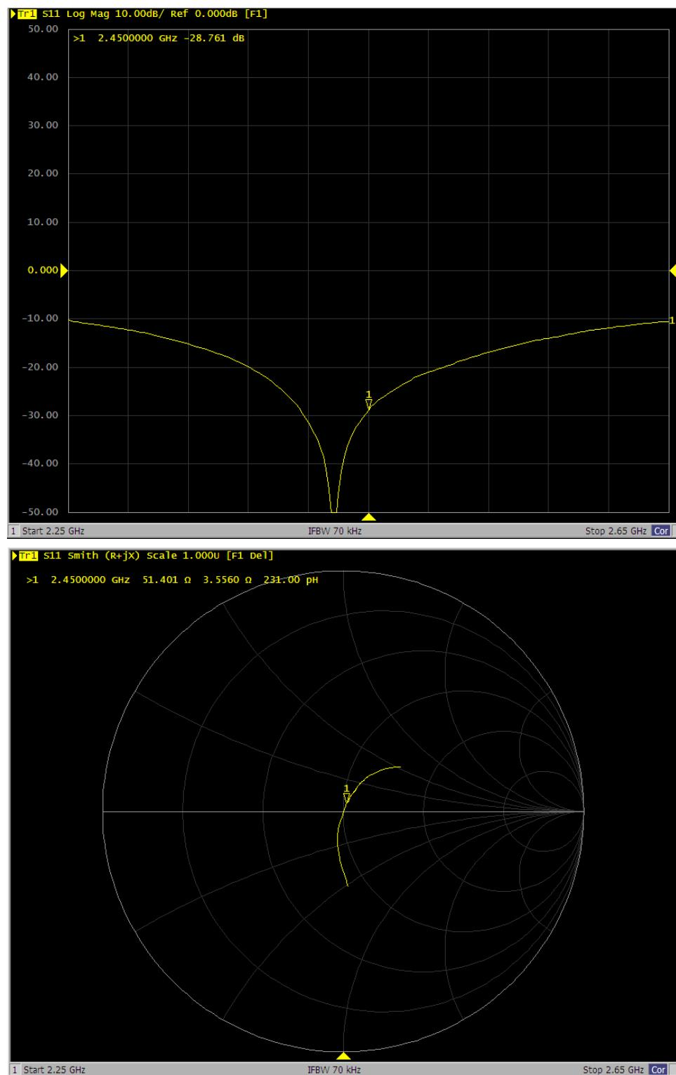
**<Dipole Verification Data> - D2450V2, serial no. 736 (Data of Measurement : 08.15.2023)**
