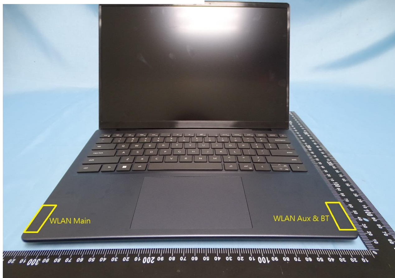
Host with Hong-BO Co., Ltd. and WNC Antenna
