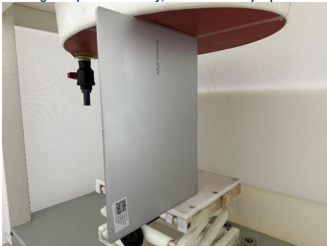
Testing Setup for Extremity, Left Side of Laptop at 0 mm
