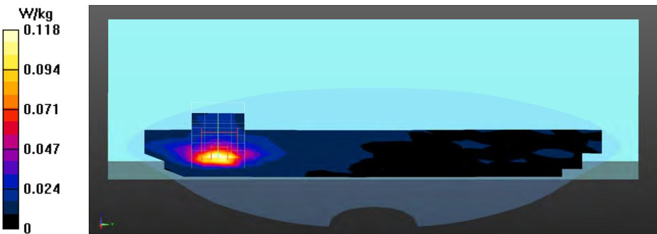
**802.11b EUT Bottom(NB) (AWAN-1 Aux(TX2) Antenna), Z-Axis plot****Channel: 1**
