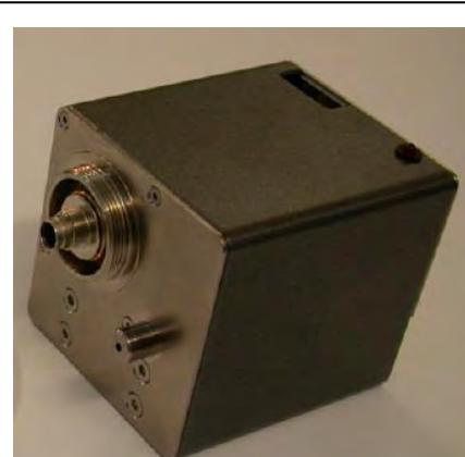
The DASY5 measurement server is based on a PC/104 CPU board with a 400MHz intel ULV Celeron, 128MB chipdisk and 128MB RAM. The necessary circuits for communication with the DAE electronics box, as well as the 16 bit AD converter system for optical detection and digital I/O interface are contained on the DASY5 I/O board, which is directly connected to the PC/104 bus of the CPU board.
