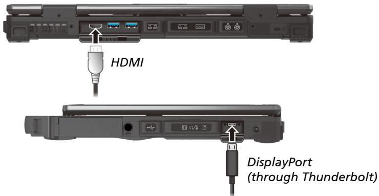
The connected device should respond by default. If not, you can switch the display output by pressing the **Fn+F5** hot keys. (You can also change the display through Windows **Control Panel**.)
