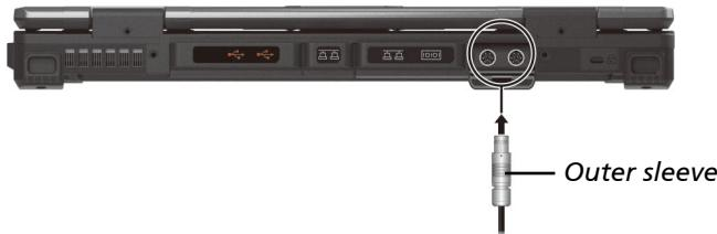
Once connected, a special locking mechanism will prevent accidental disconnection. To disconnect, push the outer sleeve to unlock and then pull the connector out.
