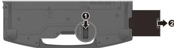
4. Noting the orientation, insert the new battery pack all the way into the bay. The battery latch should be engaged in the locked position (
