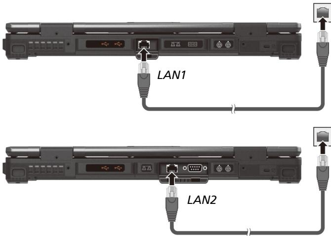
**NOTE:** LAN2 module implements DSM (Deep Slumber Mode) to save battery power. Power is supplied to the LAN module only when the LAN cable is connected. This means the LAN module will not appear in Windows' **Device Manager** if the LAN cable is not connected and will appear if the cable is connected.
