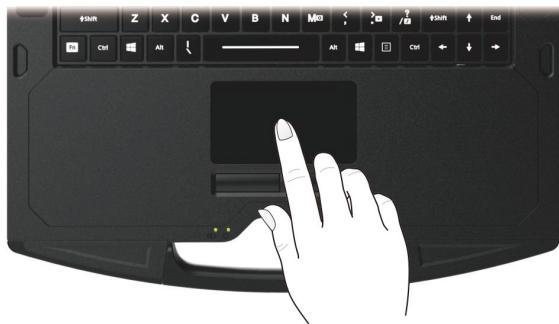
The touchpad consists of a rectangular pad (work surface) and a left and right buttons. To use the touchpad, place your forefinger or thumb on the pad. The rectangular pad acts like a miniature duplicate of your display. As you slide your fingertip across the pad, the pointer (also called cursor) on the screen moves accordingly. When your finger reaches the edge of the pad, simply relocate yourself by lifting the finger and placing it on the other side of the pad.
