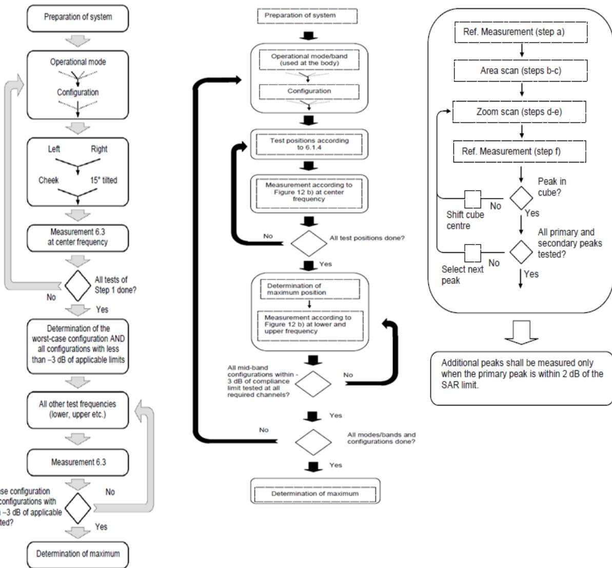
After an area scan has been done at a fixed distance of 1.4mm from the surface of the phantom on the source side, a 3D scan is set up around the location of the maximum spot SAR. First, a point within the scan area is visited by the probe and a SAR reading taken at the start of testing. At the end of testing, the probe is returned to the same point and a second reading is taken. Comparison between these start and end readings enables the power drift during measurement to be assessed.
