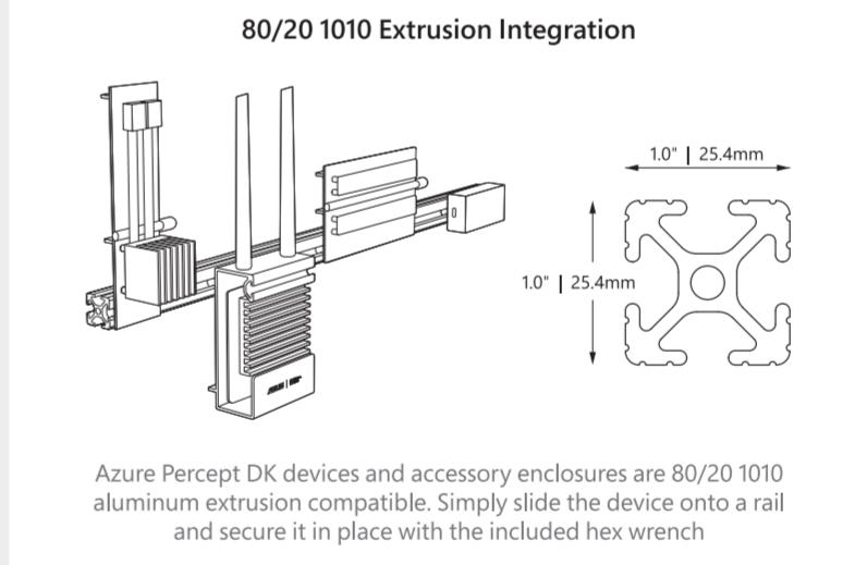
Azure Percept DK devices and accessory enclosures are 80/20 1010 aluminum extrusion compatible. Simply slide the device onto a rail and secure it in place with the included hex wrench
