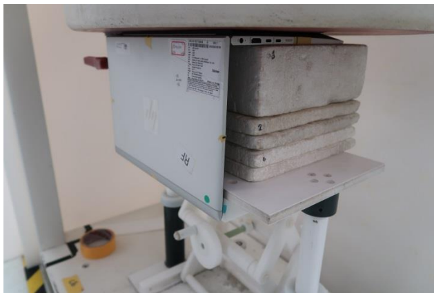
Bottom of Laptop, Test Separation 0 mm
