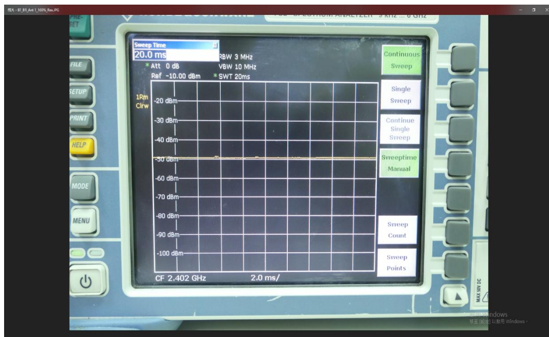
Time-domain plot for Bluetooth transmission signal
