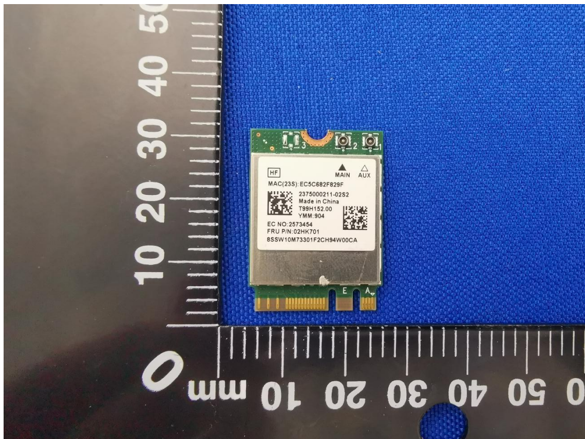
RF MODULE TOP VIEW (WITH SHIELDING)
