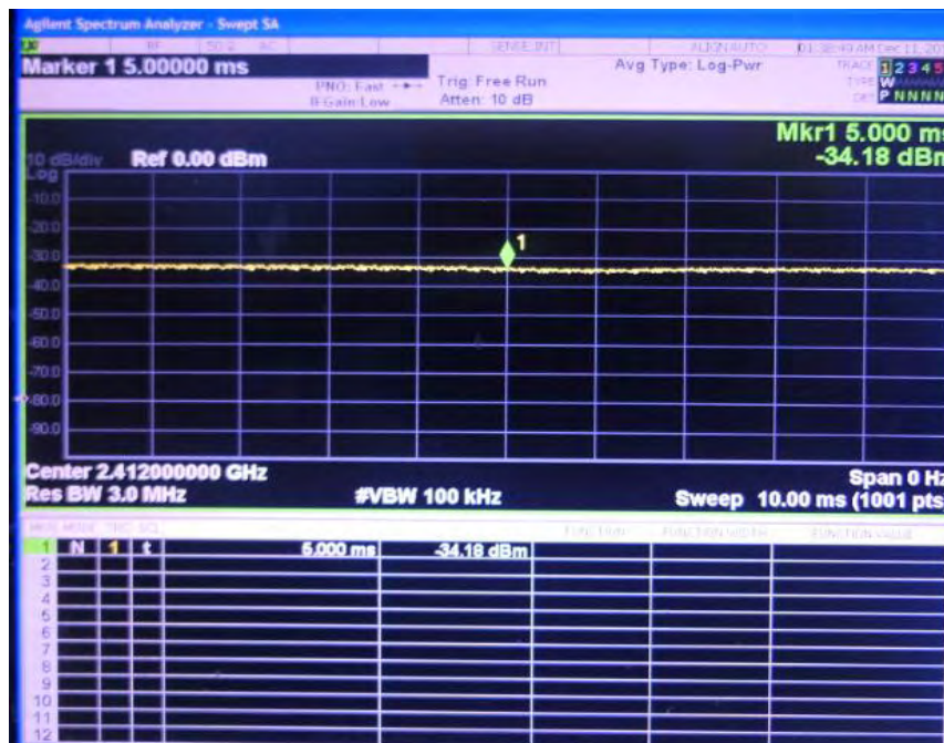
Time-domain plot for Bluetooth transmission signal
