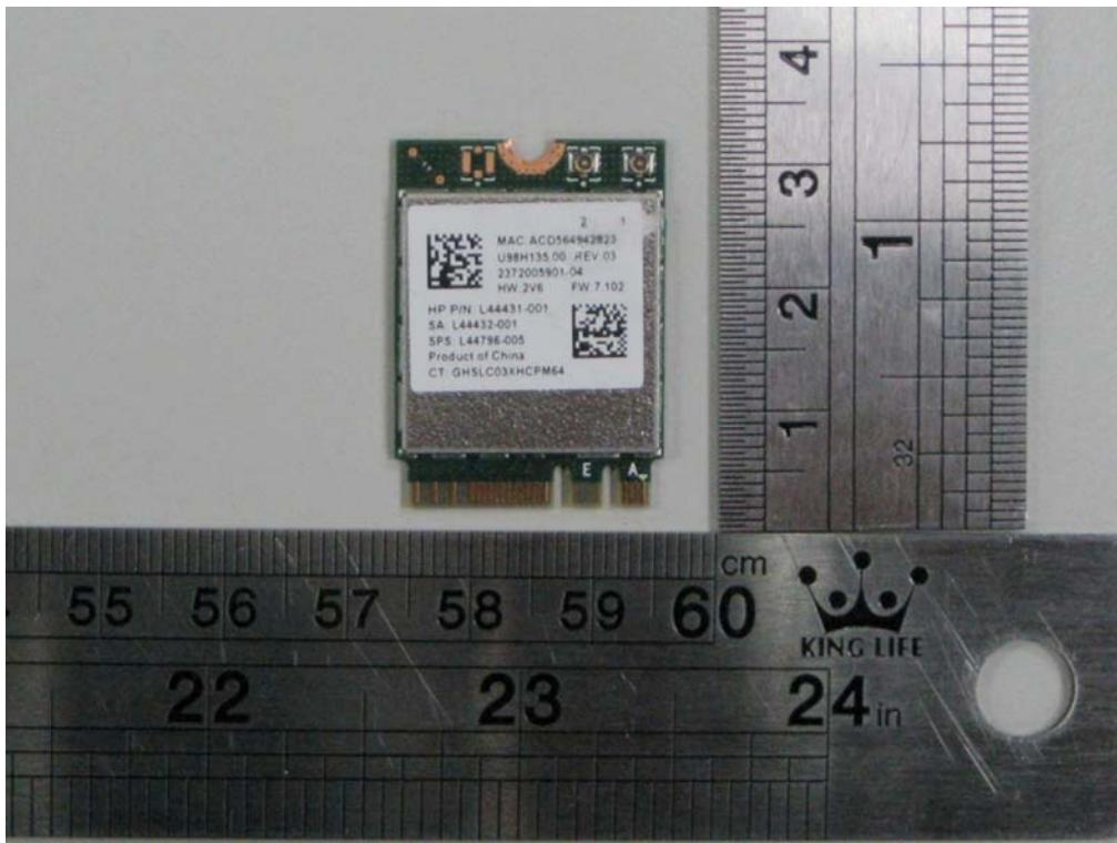
**WLAN / BT Module-2 (Model No.: RTL8822CE)**
