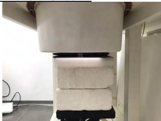
Fig.3 EUT Back side to flat phantom
