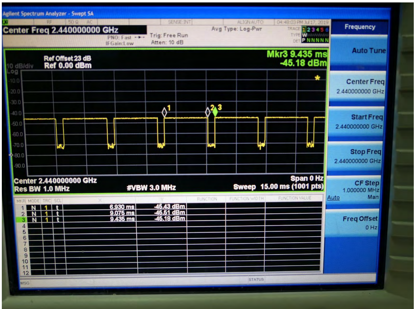
Time-domain plot for Bluetooth transmission signal
