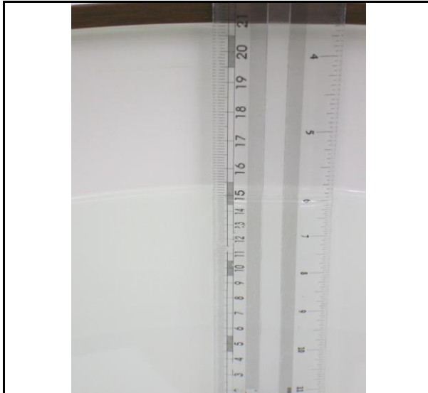
Figure 5. Liquid Height for Body SAR
