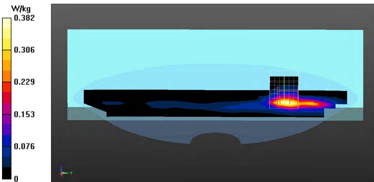
**802.11b\_Bottom-Aux-WGT Antenna, Z-Axis plot****Channel: 6**
