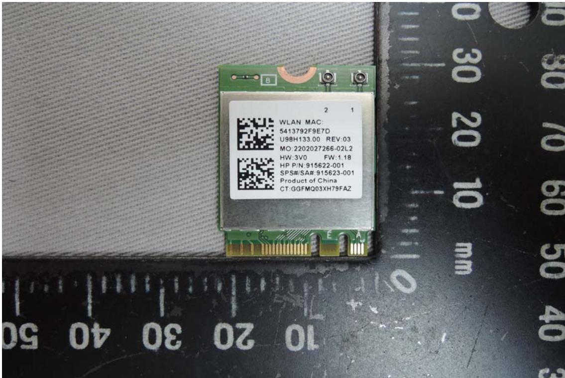
***WLAN / BT Module - 2 (Model No.: RTL8822BE)***
