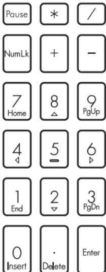
A numeric keypad is available on selected Notebook PC models. You can use this keypad for numeric input or as pointer direction keys.
