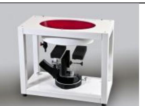
A photograph of the ELI Phantom. It is a white rectangular phantom with a red circular top. The top cover is removed, showing the internal structure and the device holder. |
