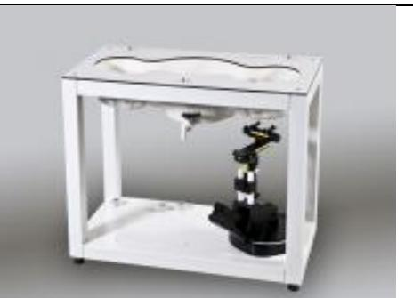
A photograph of the SAM Twin Phantom. It is a white rectangular phantom with a black device holder inside. The top cover is removed, showing the internal structure and the device holder. |
