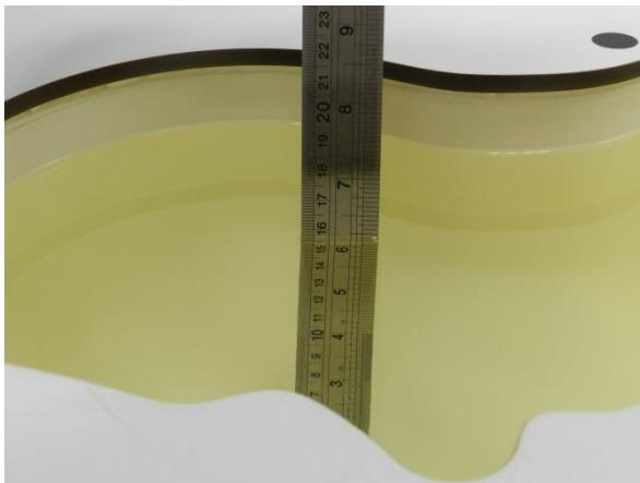
Fig 10.1 Photo of Liquid Height for Head SAR
