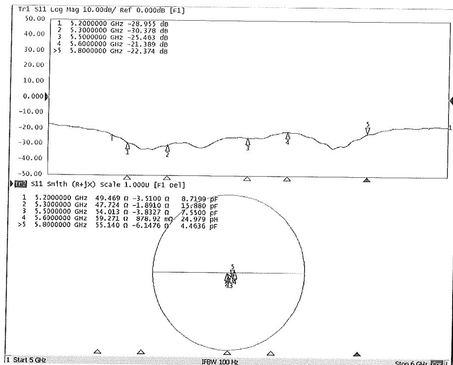
**D5GHzV2, Serial No.1095 Extended Dipole Calibrations**
