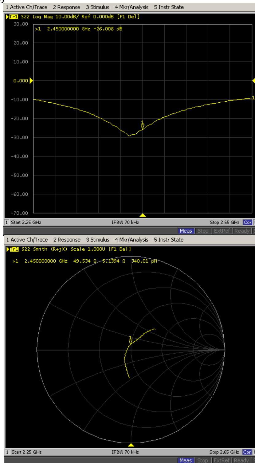
**D2450V2, Serial No.817 Extended Dipole Calibrations**
