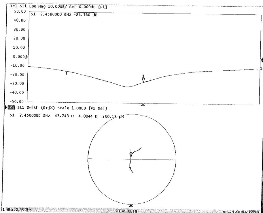
**D2450V2, Serial No.817 Extended Dipole Calibrations**
