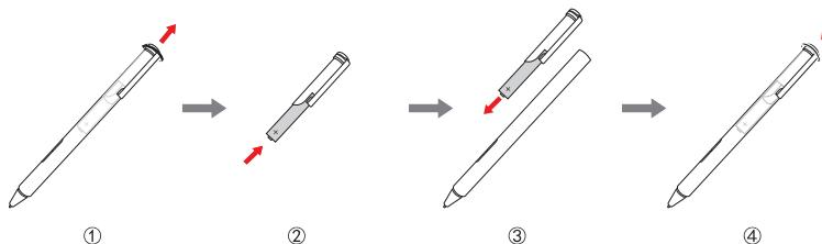
**Note:** Insert the battery by matching the + and – terminals on the battery to the + and – terminals in the battery compartment.
