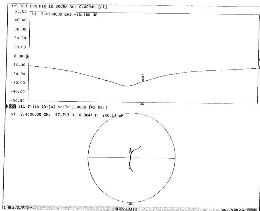
**D2450V2, Serial No.817 Extended Dipole Calibrations**
