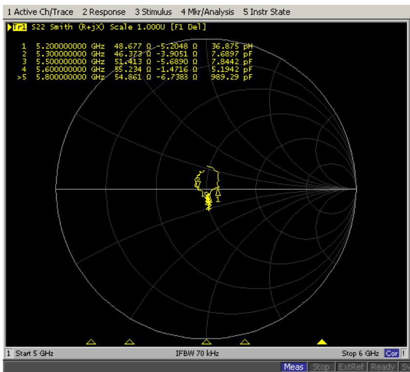
**Dipole Verification Data D5GHzV2 Serial No.1095**
