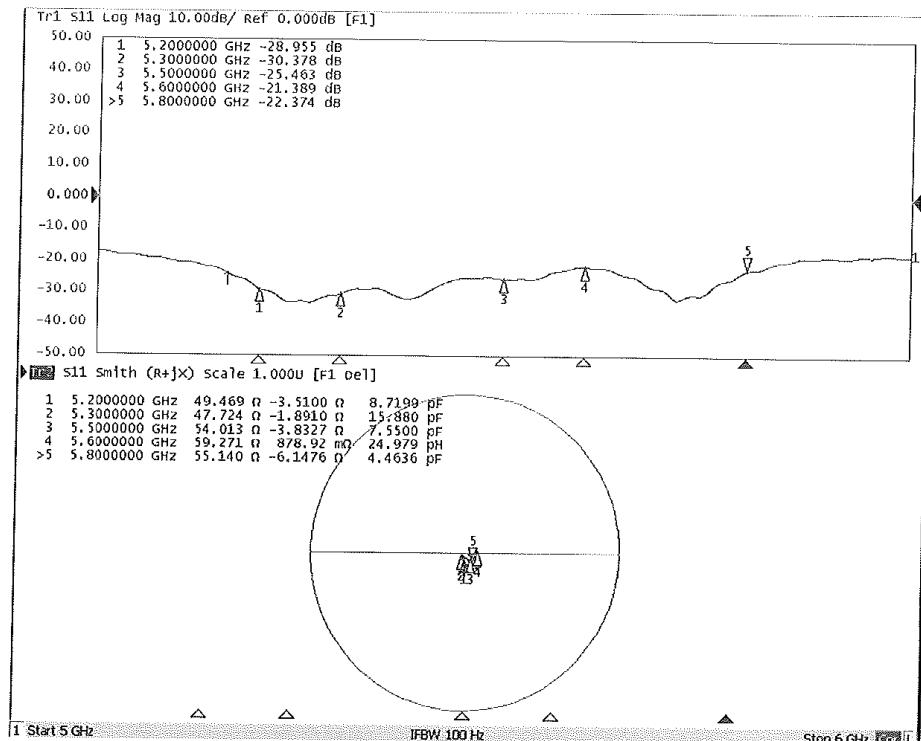
**D5GHzV2,Serial No.1095 Extended Dipole Calibrations**
