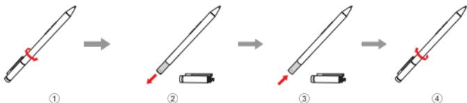
**Note:** Insert the battery by matching the + and – terminals on the battery to the + and – terminals in the battery compartment.
