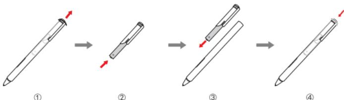
**Note:** Insert the battery by matching the + and – terminals on the battery to the + and – terminals in the battery compartment.
