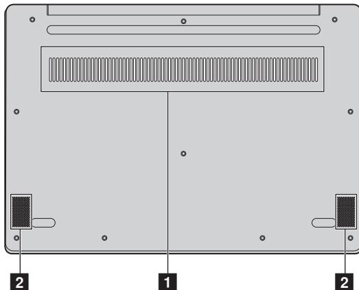
**1 Ventilation slots** Dissipate internal heat.
