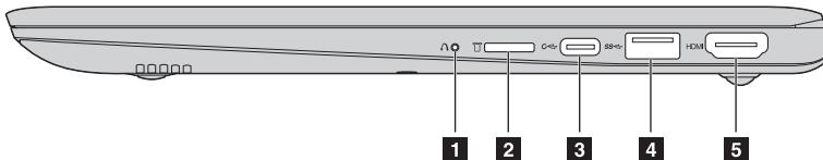
**1 Novo button** When the computer is off, press this button to start the System Recovery or the BIOS setup utility, or to enter the boot menu.
