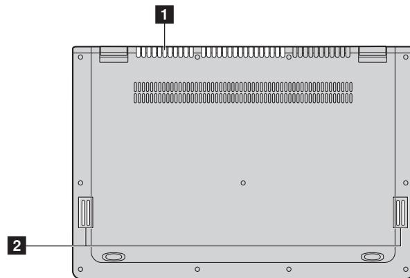
**1 Ventilation slots** Allow air to enter the computer for cooling.
