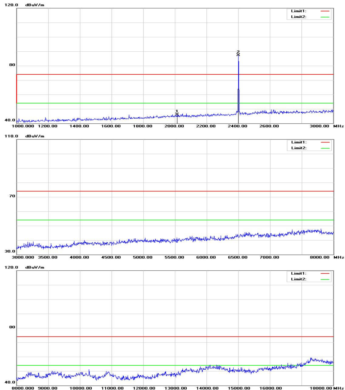
**Above 1 GHz****Operation Mode:** TX / GFSK / DH5 / CH Low**Test Date:** August 1, 2015**Temperature:** 27°C**Tested by:** Jason Lu**Humidity:** 53 % RH**Polarity:** Ver. / Hor.
