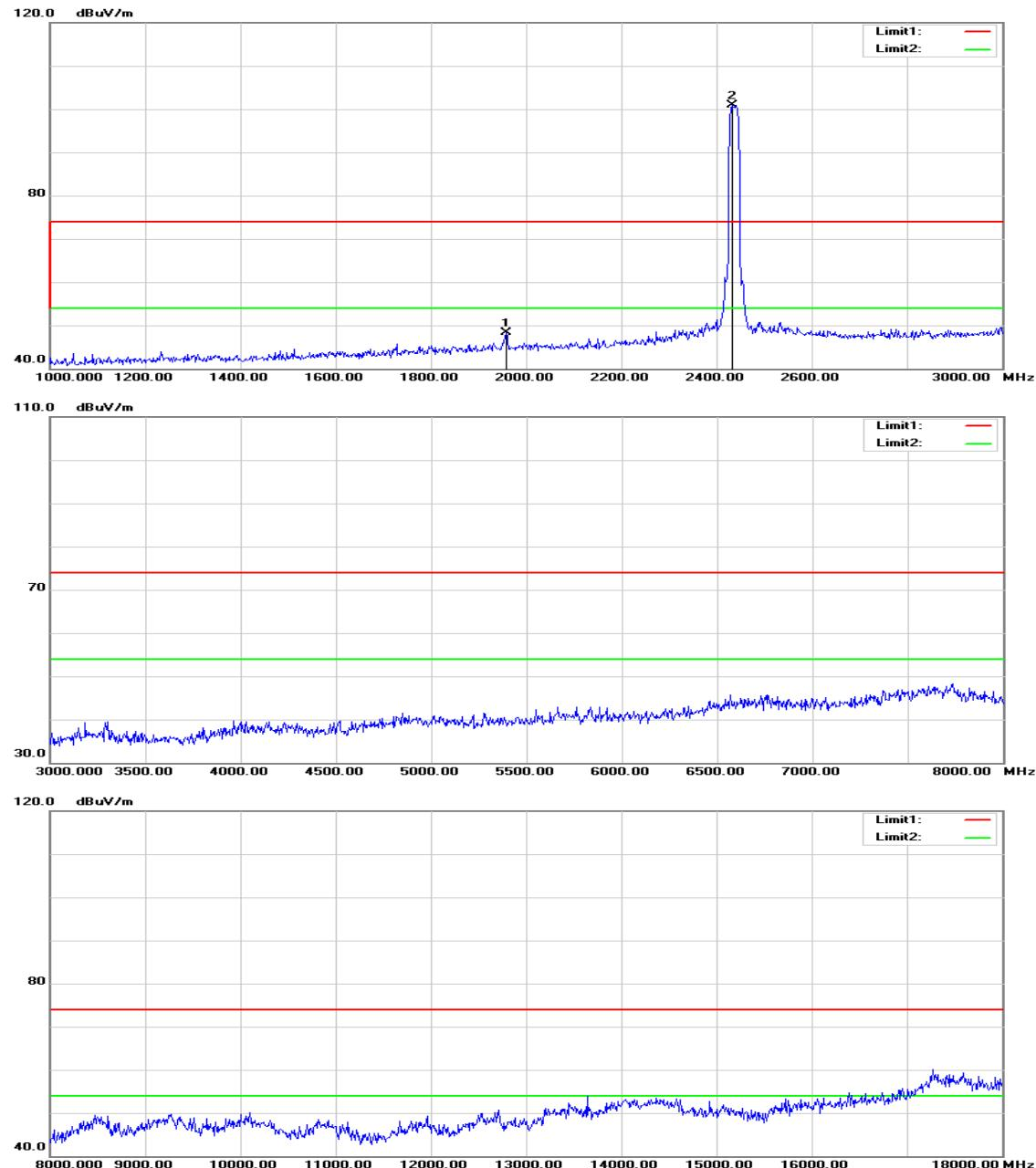
**Operation Mode:** TX / IEEE 802.11g / CH Mid**Test Date:** August 2, 2015**Temperature:** 27°C**Tested by:** Jason Lu**Humidity:** 53% RH**Polarity:** Ver. / Hor.
