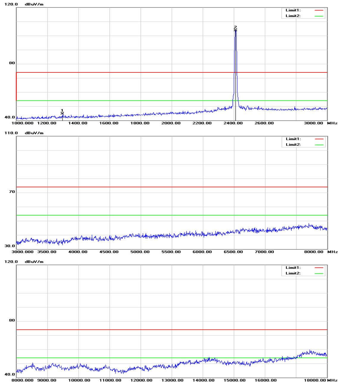
**Above 1 GHz****Operation Mode:** TX / IEEE 802.11b / CH Low**Test Date:** August 2, 2015**Temperature:** 27°C**Tested by:** Jason Lu**Humidity:** 53% RH**Polarity:** Ver. / Hor.
