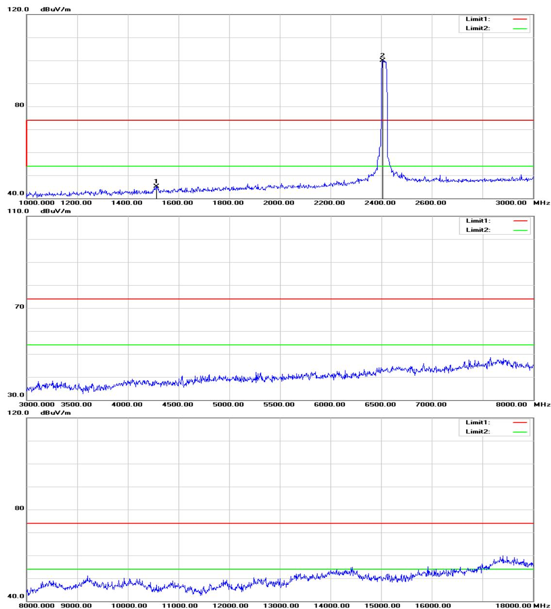
**Operation Mode:** TX / IEEE 802.11n HT 20 MHz mode / CH Low **Test Date:** August 2, 2015
