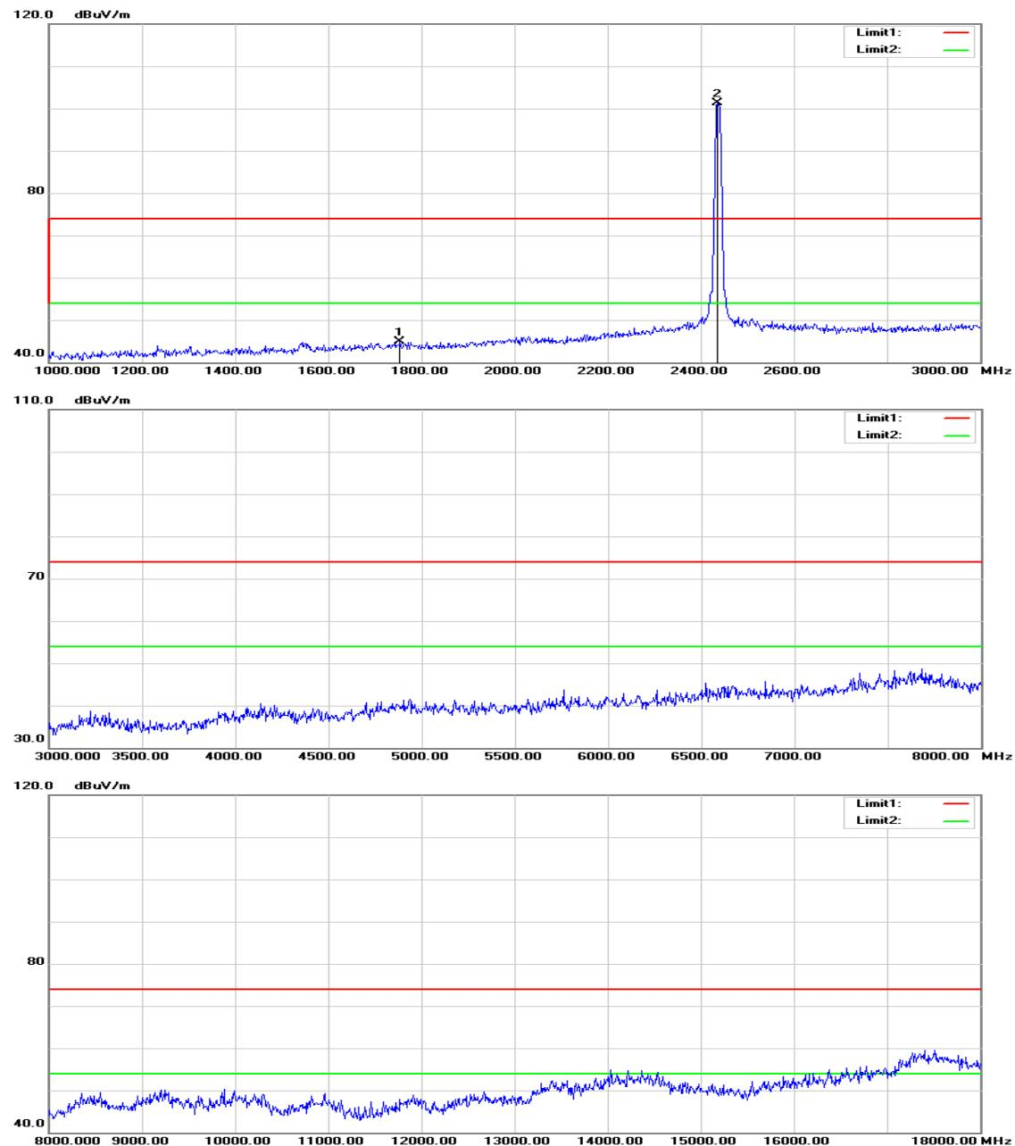
**Operation Mode:** TX / IEEE 802.11b / CH Mid**Test Date:** August 2, 2015**Temperature:** 27°C**Tested by:** Jason Lu**Humidity:** 53% RH**Polarity:** Ver. / Hor.
