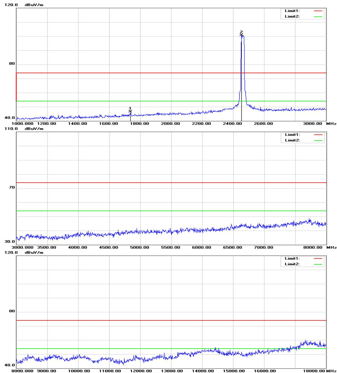
**Operation Mode:** TX / IEEE 802.11g / CH High**Test Date:** August 2, 2015**Temperature:** 27°C**Tested by:** Jason Lu**Humidity:** 53% RH**Polarity:** Ver. / Hor.
