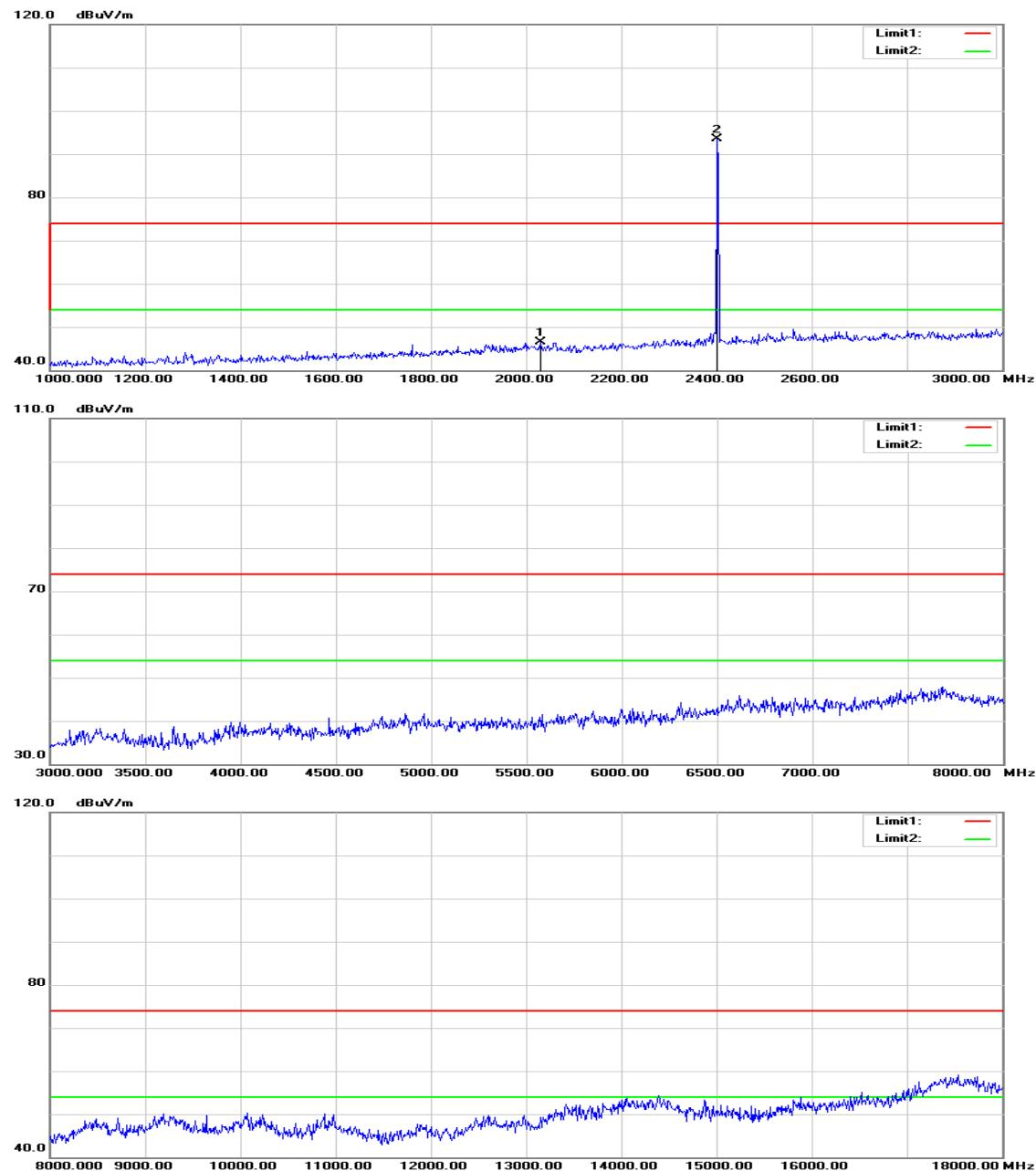
**Operation Mode:** GFSK / TX / CH Low **Test Date:** August 1, 2015
