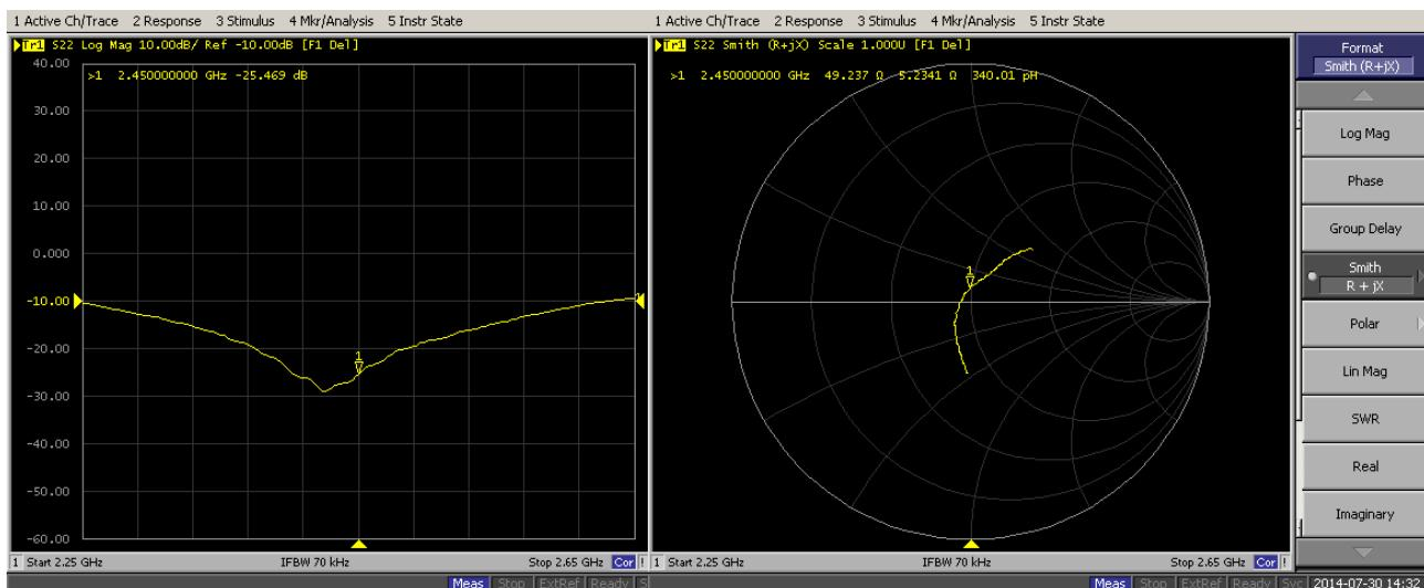
Per IEEE Std 1528-2003, the dipole should have a return loss better than -20dB at the test frequency to reduce uncertainty in the power measurement.
