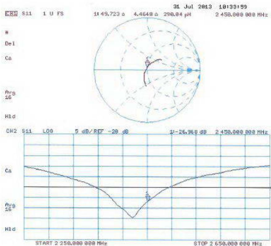
**D2450V2, Serial No.817 Extended Dipole Calibrations**
