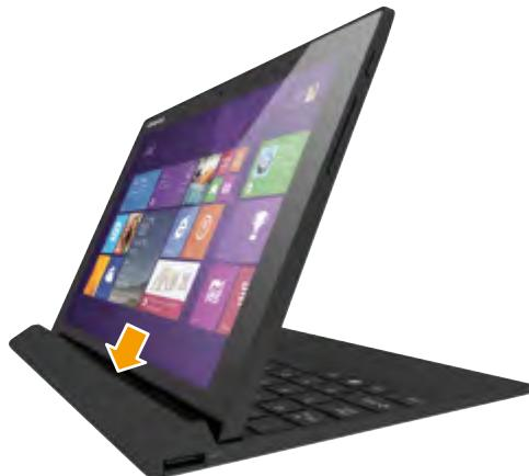
**Detaching the tablet:** Remove the tablet in the direction shown by the arrow.
