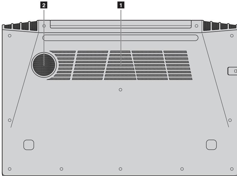
**1 Louvers** Allow air to enter the computer for cooling.
