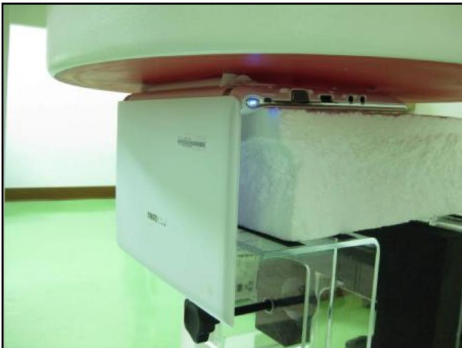
The bottom of the notebook contacts the bottom of the flat phantom with 0mm-separation distance.
