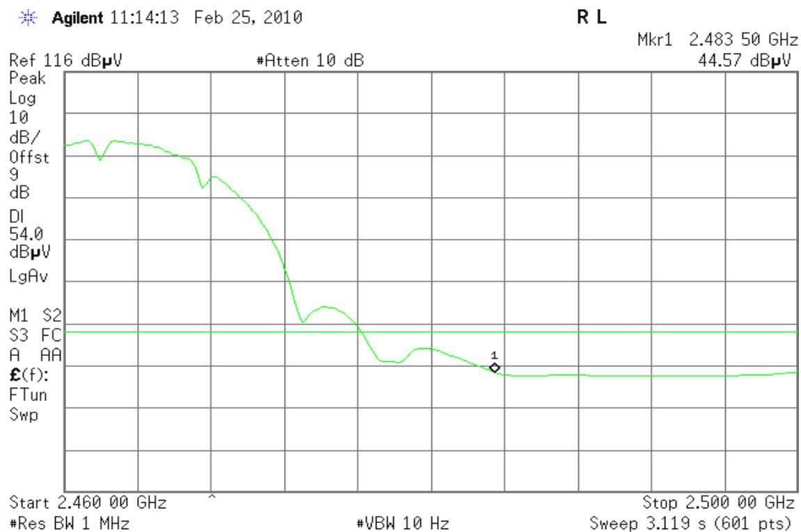
**Band Edges (IEEE 802.11g mode / CH Low)****Detector mode: Peak****Polarity: Vertical**
