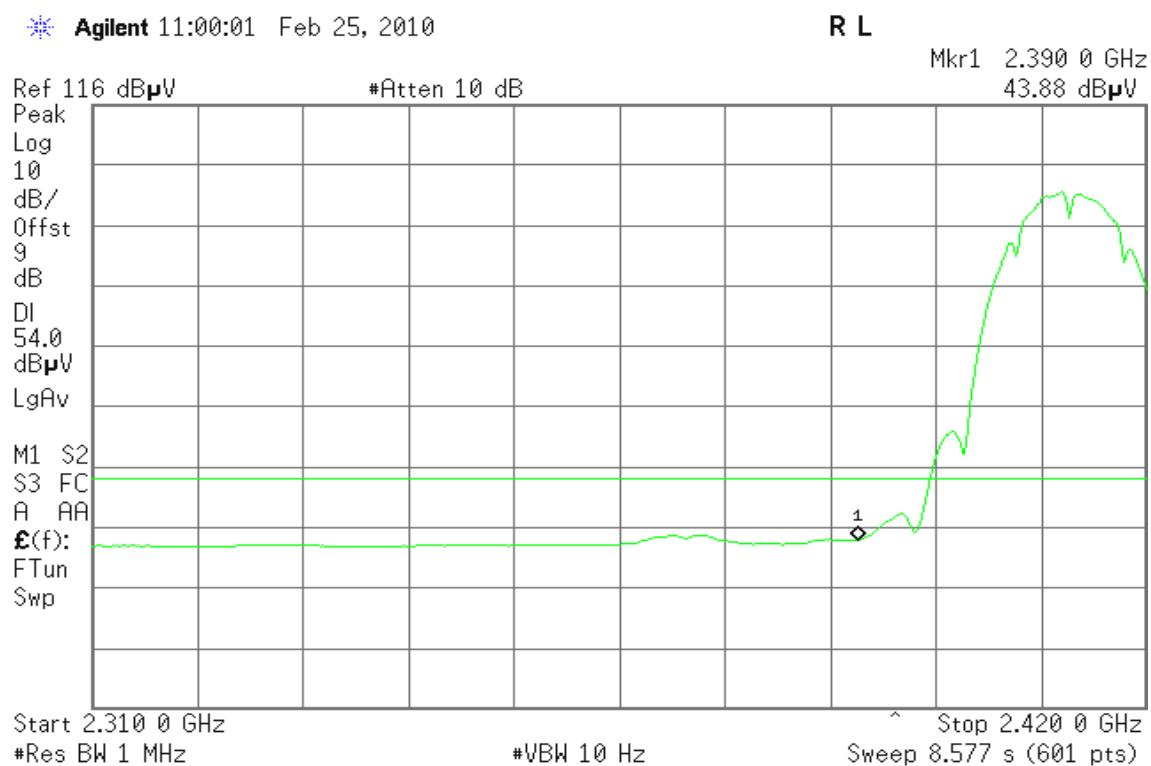
**Band Edges (IEEE 802.11b mode / CH High)****Detector mode: Peak****Polarity: Vertical**
