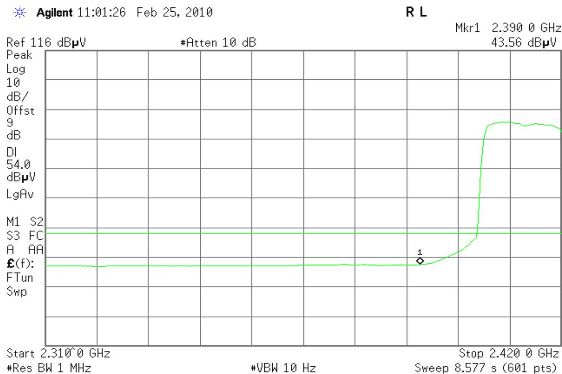
**Band Edges (IEEE 802.11g mode / CH High)****Detector mode: Peak****Polarity: Vertical**
