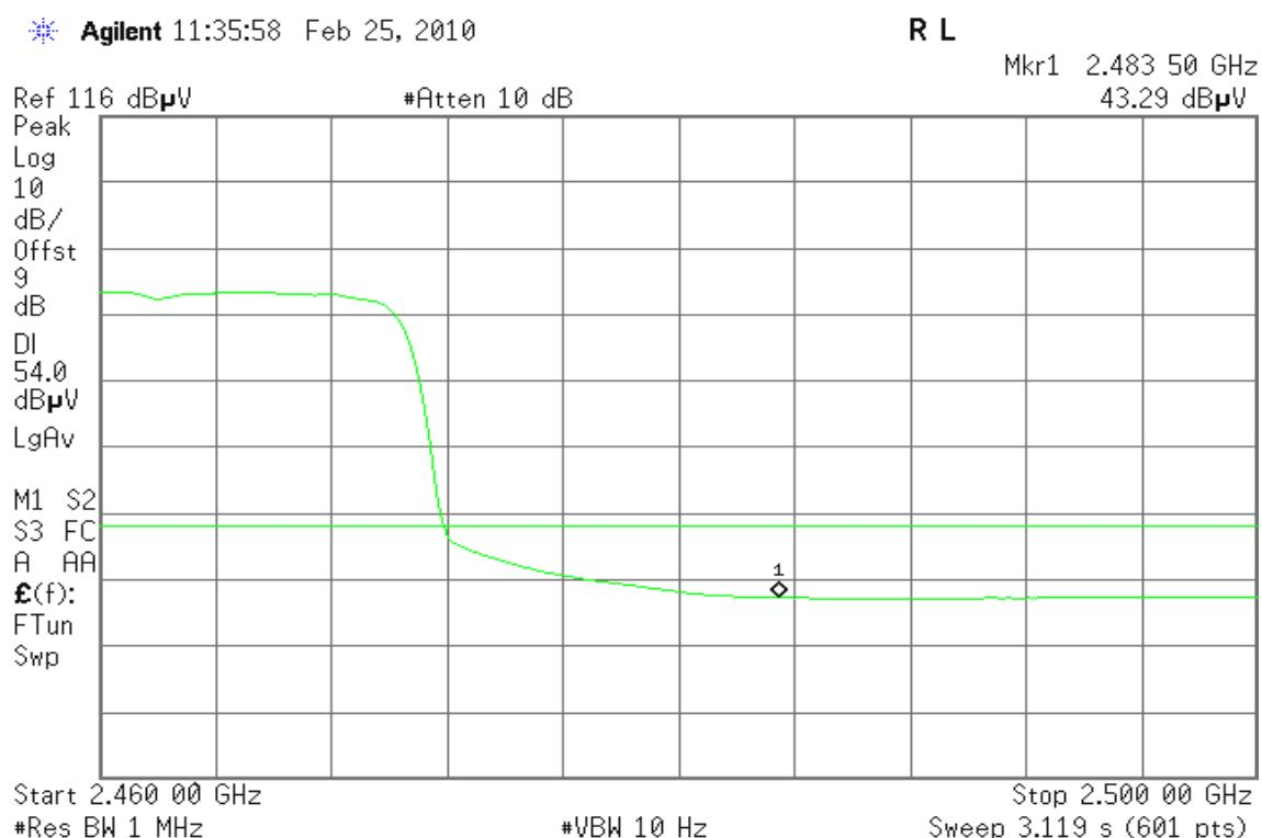
**Detector mode: Peak****Polarity: Horizontal**
