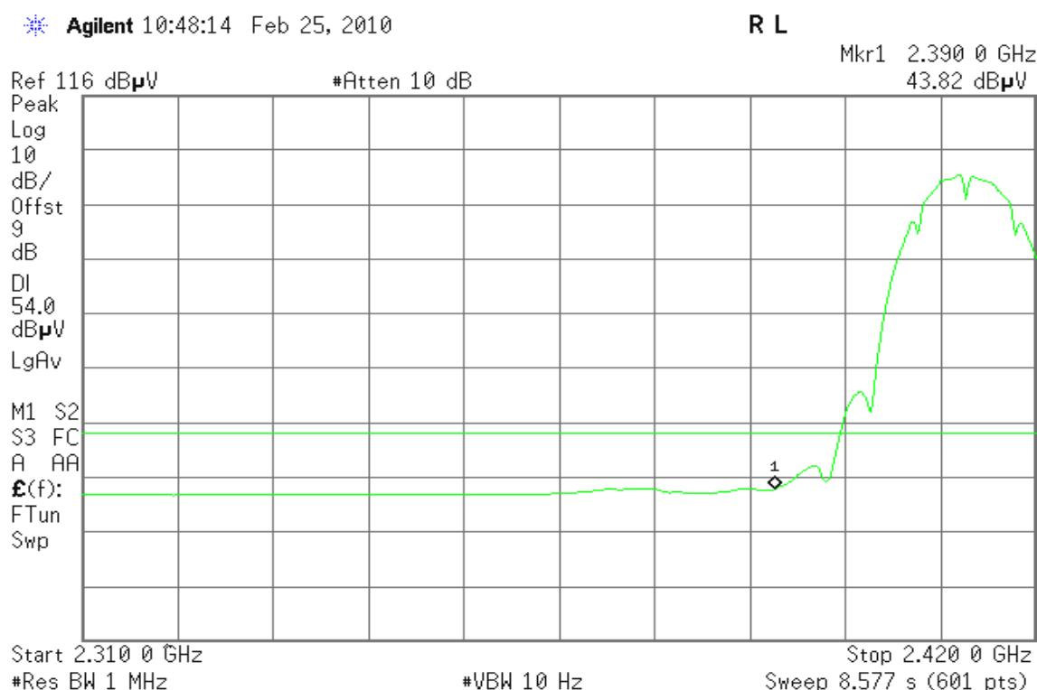
**Detector mode: Peak****Polarity: Horizontal**
