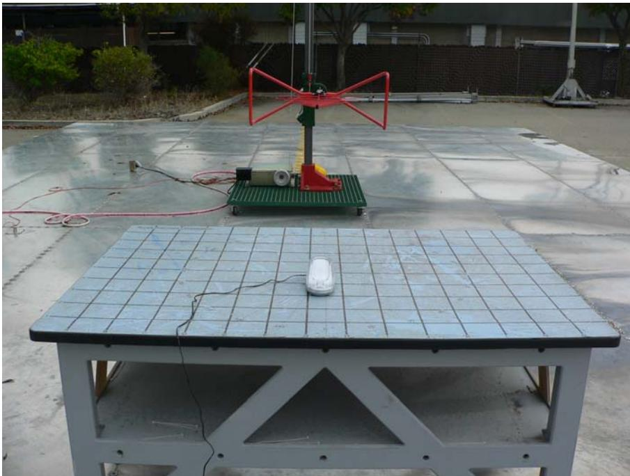
**Base of EUT: Radiated Emission - Rear View**
