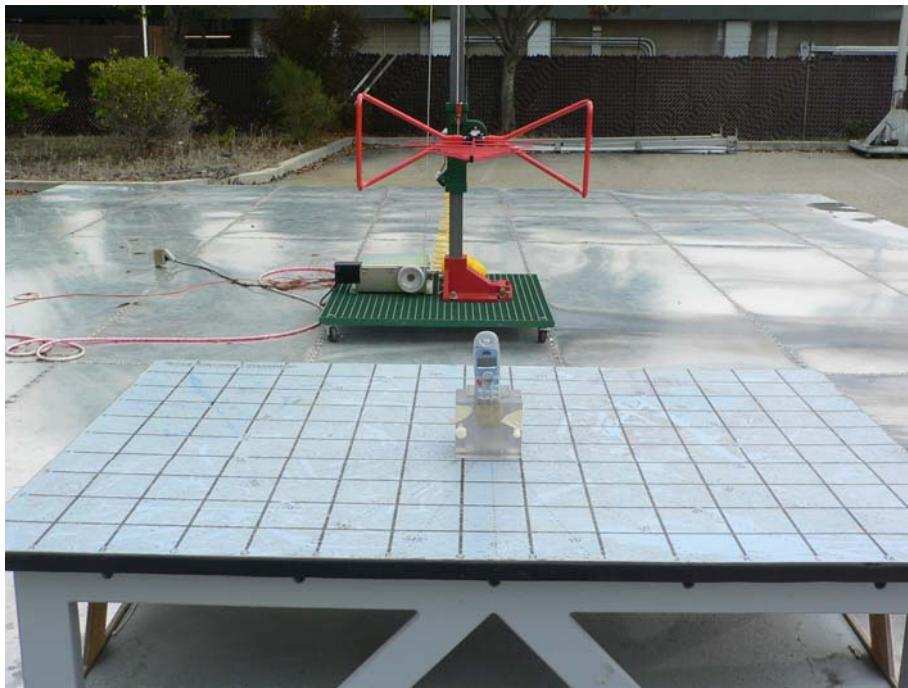
**Handset of EUT: Radiated Emission - Rear View**
