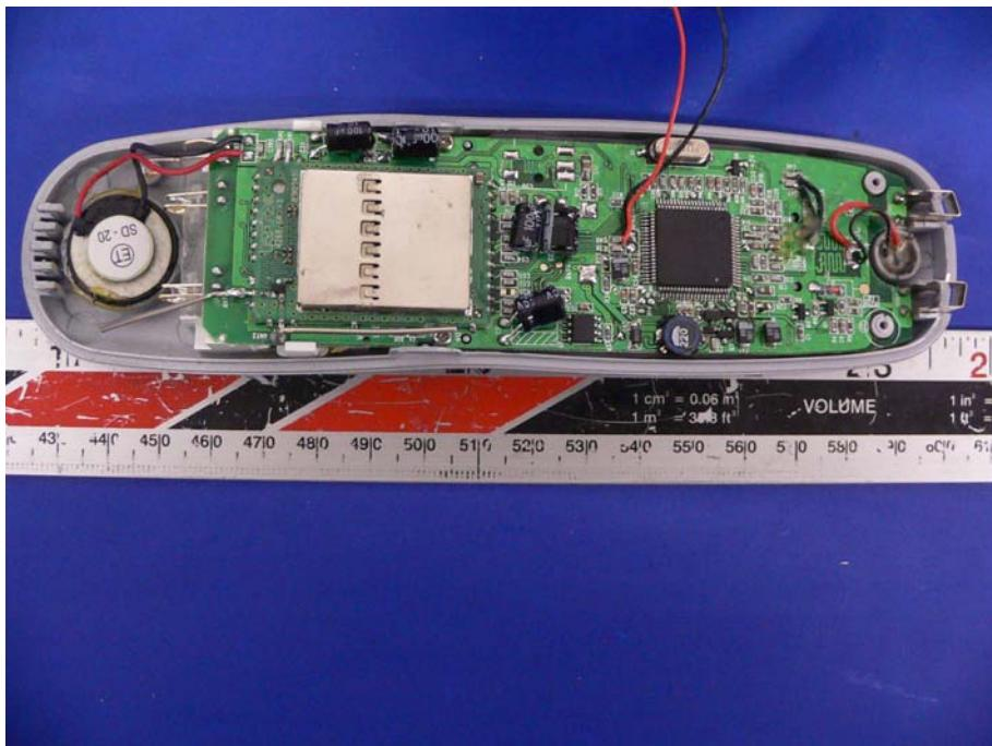
**Handset of EUT: EUT –Component View**
