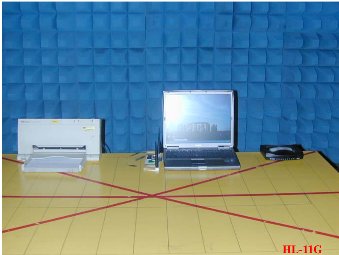
Photo 1: Radiated Emission Test Set-up
