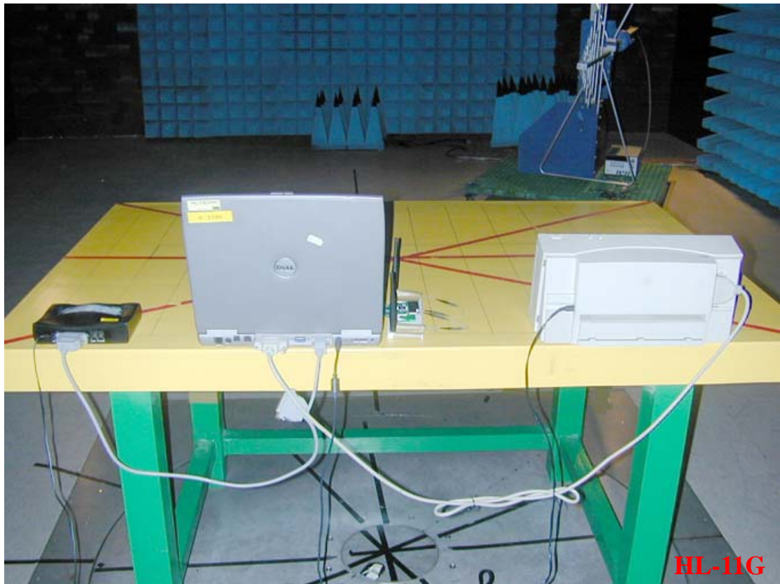
Photo 2: Radiated Emission Test Set-up
