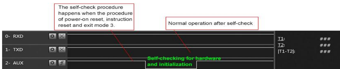
Timing Sequence Diagram of AUX when self-check
