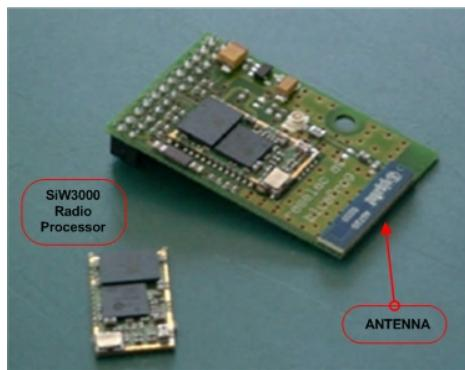
The Bluetooth module is a class 2 (0 dBm) module. The module based on the RF Micro Devices SiW3000™ Radio Processor which combines the ARM7TDMI processor for Bluetooth wireless technology.
