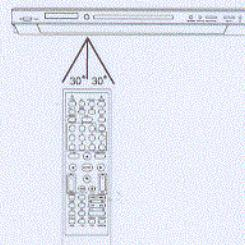
**Distance :** within 7m from the front of the remote control sensor.
