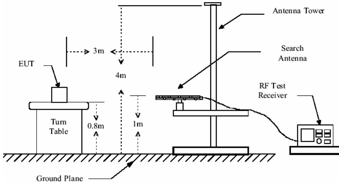
The field strength is calculated by adding the Antenna Factor, Cable Factor & Peramplifier .
