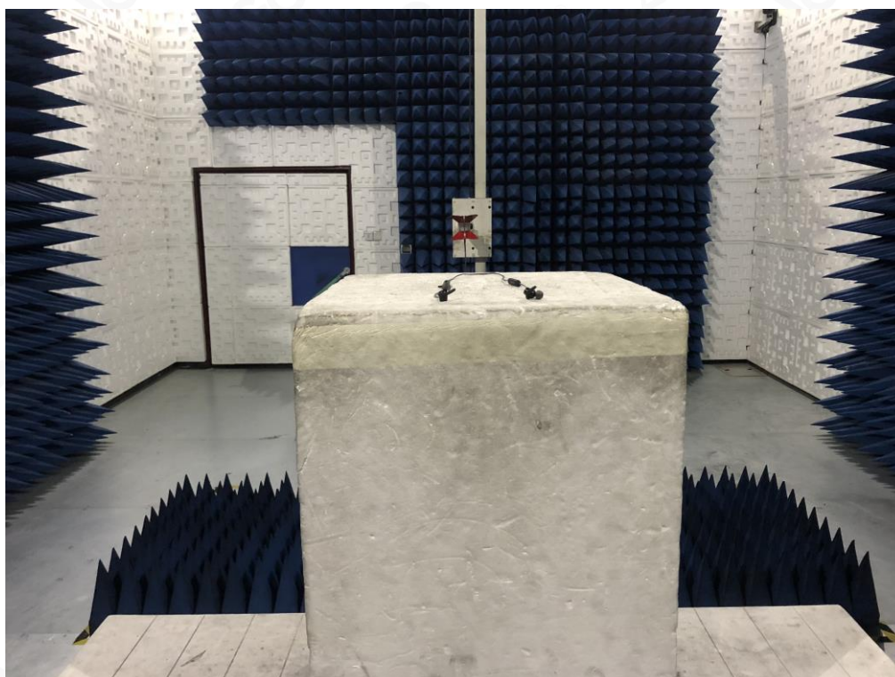
RADIATED EMISSION TEST SETUP ABOVE 1GHZ
