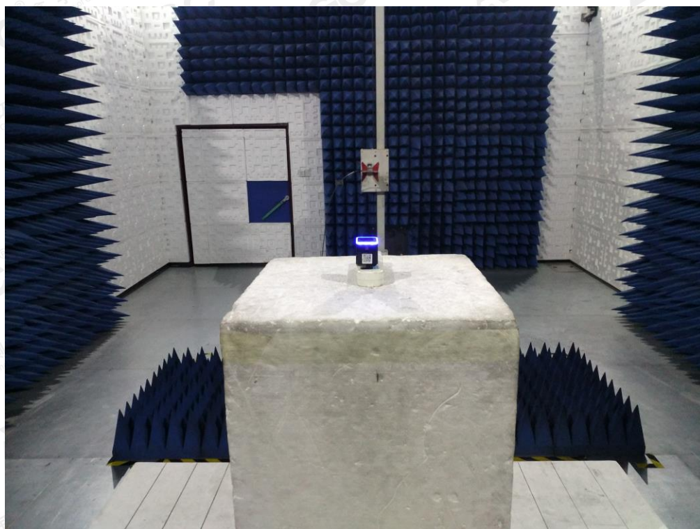
FCC RADIATED EMISSION TEST SETUP ABOVE 1GHZ
