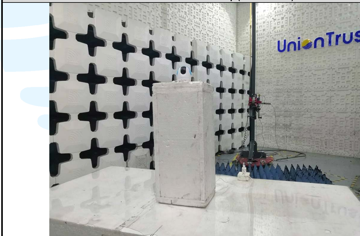
Radiated emission Test Setup (Above 1 GHz)
