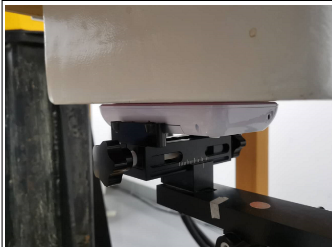
Front Face 0° of EUT with 0 cm Gap
