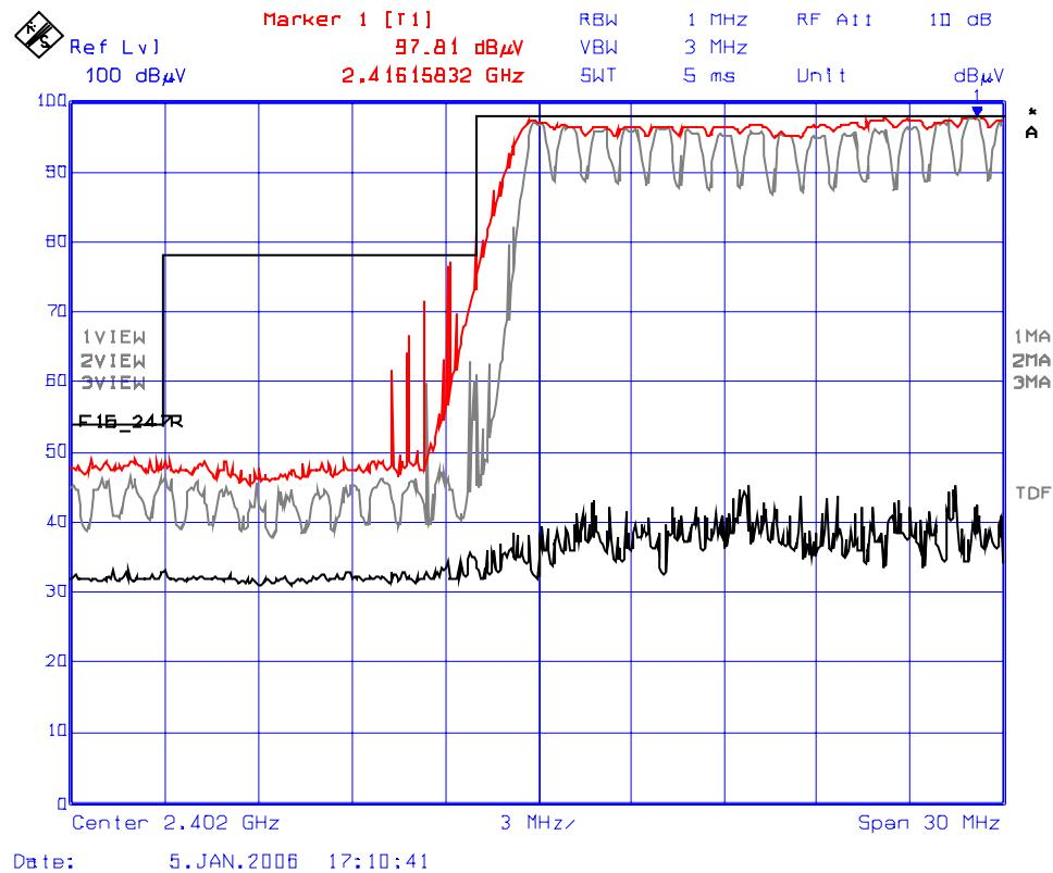
**Plot #14: Lower Band-Edge Radiated Emissions, Hopping Mode, Vertical Polarization**
