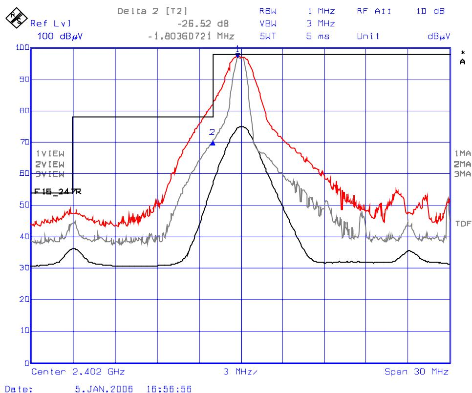
**Plot #11: Lower Band-Edge Radiated Emissions, Continuous Mode, Vertical Polarization**
