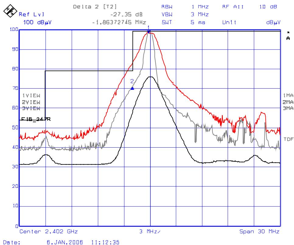
**Plot #13: Lower Band-Edge Radiated Emissions, Hopping Mode, Horizontal Polarization**
