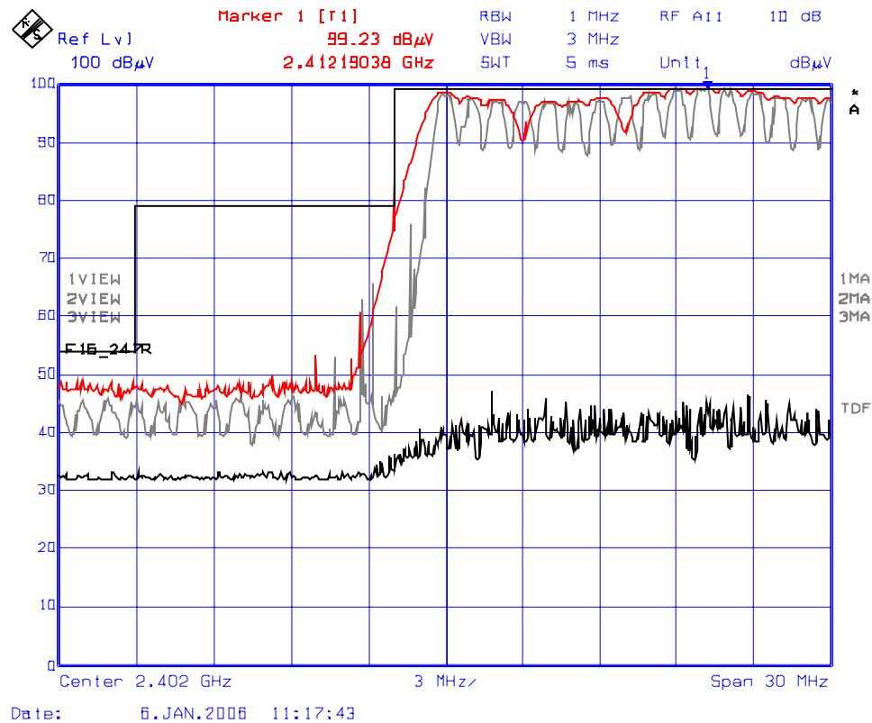
**Plot #15: Upper Band-Edge Radiated Emissions, Continuous Mode, Horizontal Polarization**
