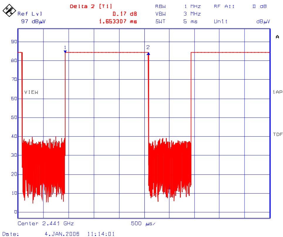
Plot #8: Pulse Train (39 pulses) in 100 mS Interval
