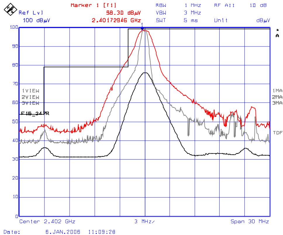
**Plot #12: Lower Band-Edge Radiated Emissions, Continuous Mode, Vertical Polarization**
