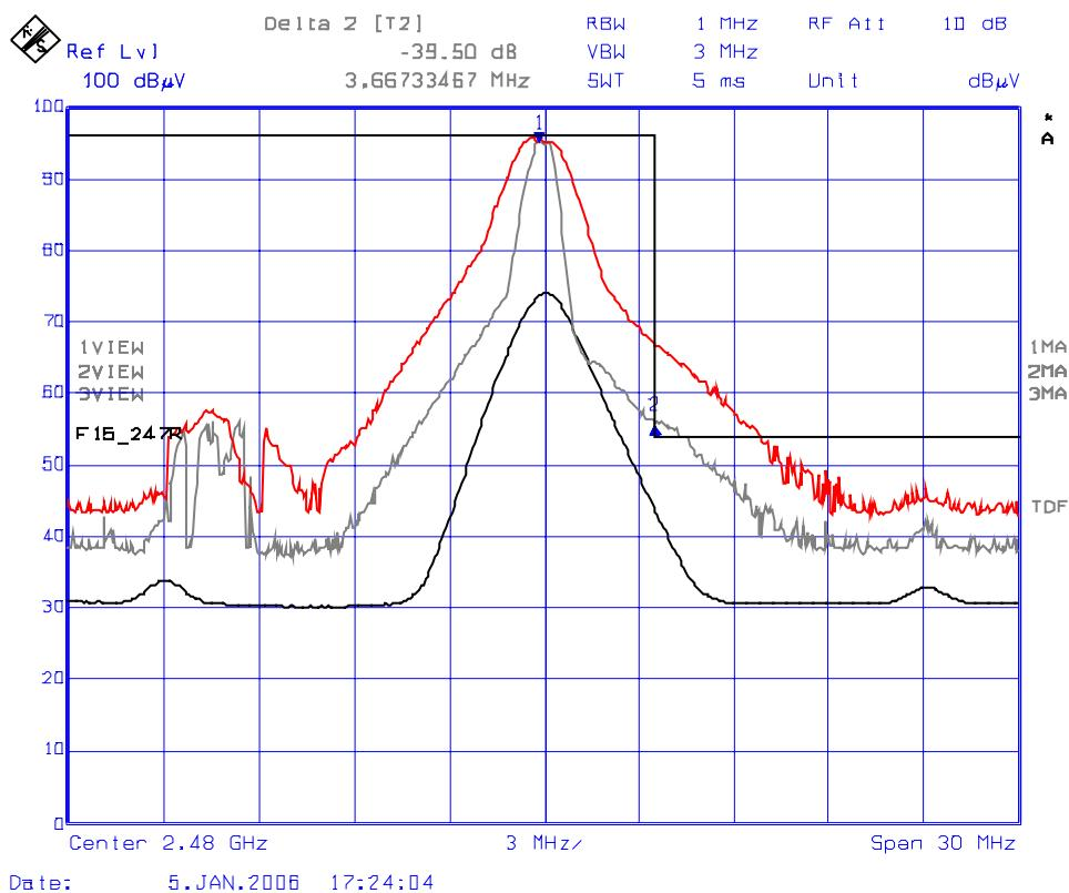
**Plot #17: Upper Band-Edge Radiated Emissions, Continuous Mode, Vertical Polarization**
