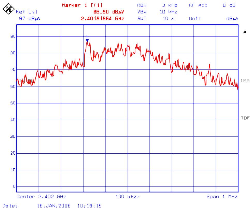
Plot #22: Power Spectral Density in 3 KHz, Frequency: 2441 MHz
