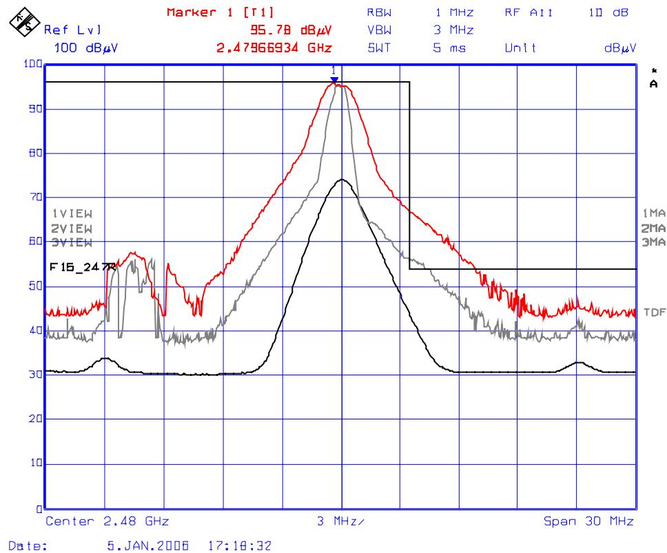
**Plot #16: Upper Band-Edge Radiated Emissions, Continuous Mode, Horizontal Polarization**
