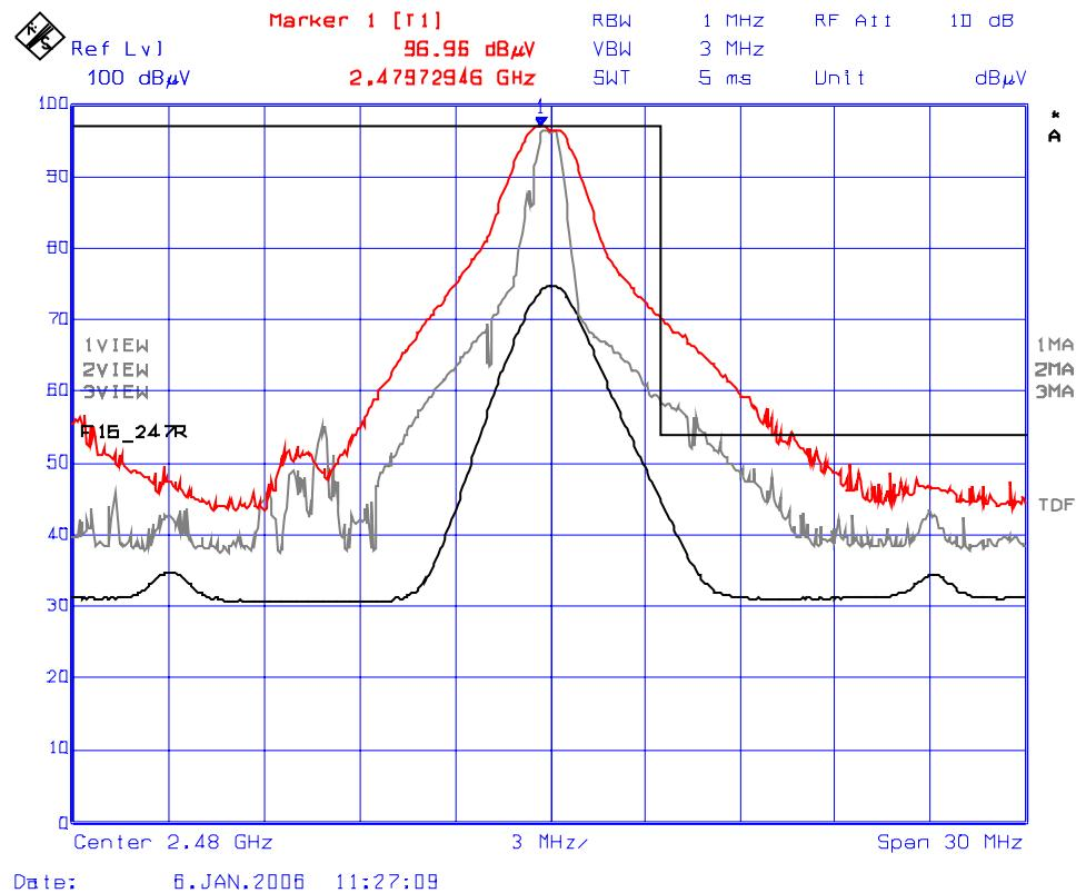
**Plot #18: Upper Band-Edge Radiated Emissions, Continuous Mode, Vertical Polarization**
