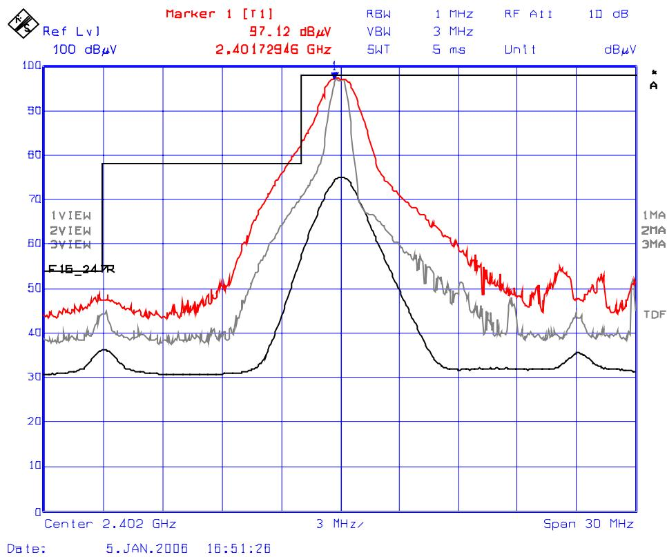
**Plot #10: Lower Band-Edge Radiated Emissions, Continuous Mode, Horizontal Polarization**
