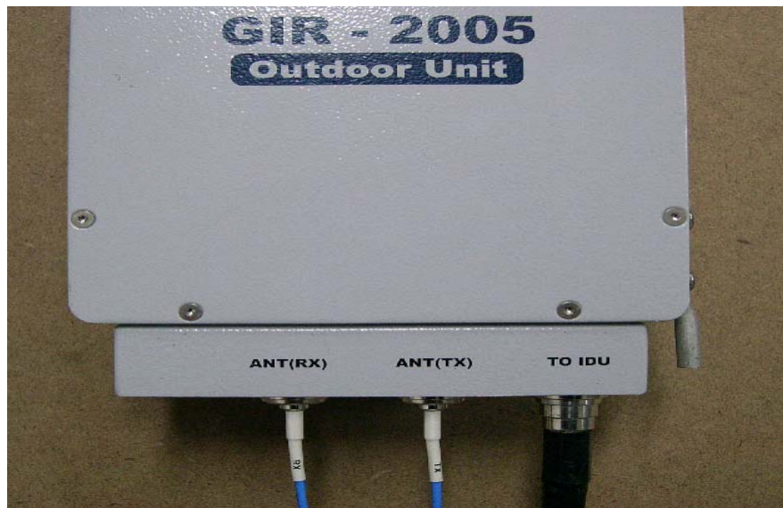
Figure 3-5 ODU connected to IDU & Internal Antenna using cables
