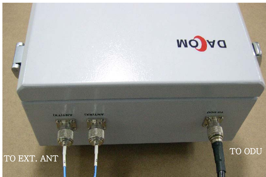
Figure 3-6 IDU connected to ODU & External Antenna using cables
