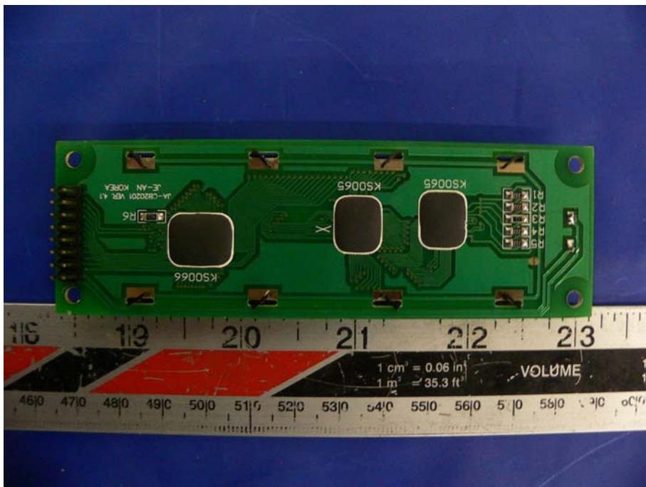
**EUT- Keypad Unit Main board Component View**
